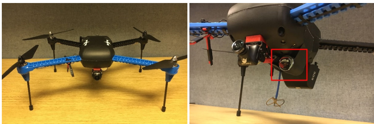
Figure 7.7-1: 3D Robotics IRIS+, Shown in Heavy Loading Configuration with 200-Gram Payload.
